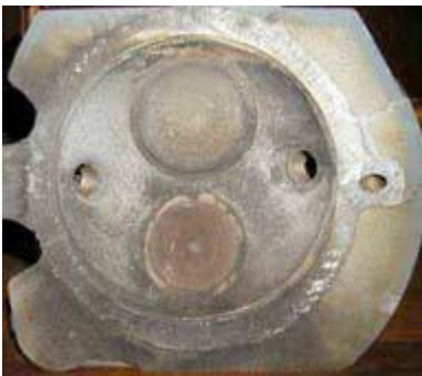
A cracked cylinder head
